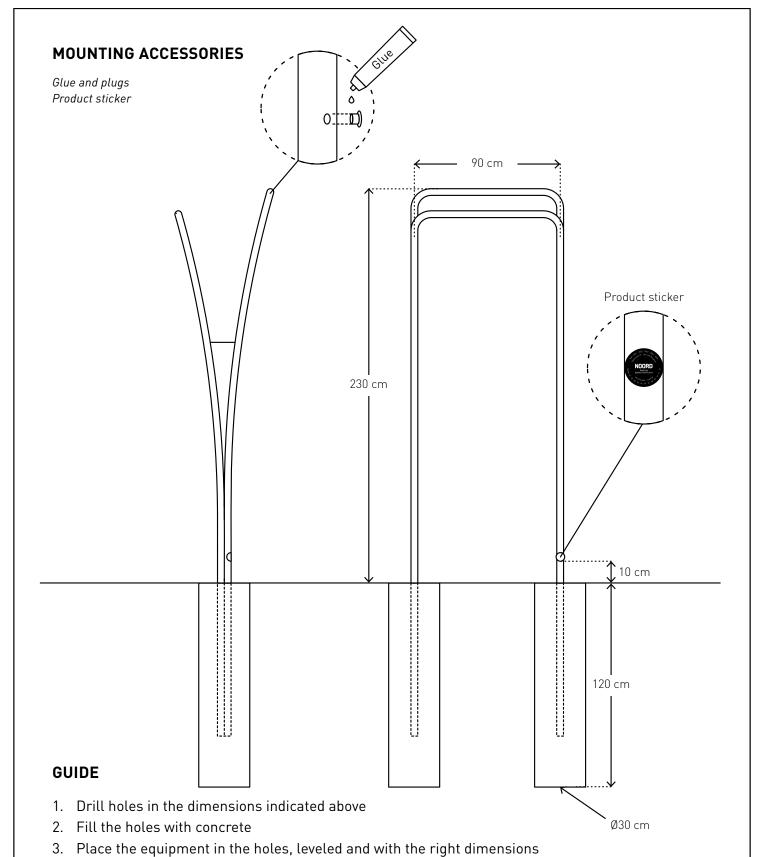
Glue the plugs into the holes in the equipment and place the product sticker as shown above
